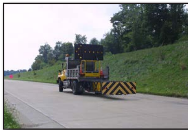
Figure 8.7 – Most transportation agencies have barrier vehicles suited for lengthy deployments.
