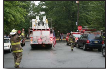
Figure 7.12 – Use at least one backer when the apparatus is being moved in reverse. (Photo/Ron Jeffers, Union City, New Jersey)
